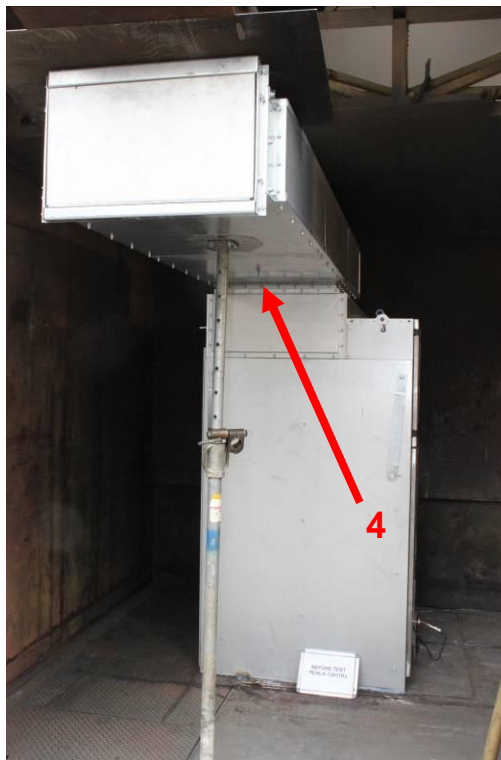
Photo No. 06 Before test PEHLA 13031Ra / 06 Test object, side view with pressure sensor 4
