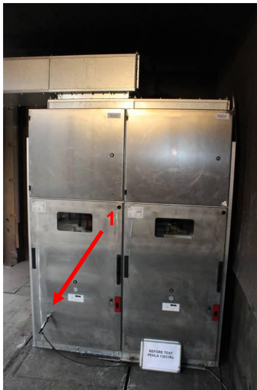
Photo No. 04 Before test PEHLA 13031Ra / 06 Test object, front view with pressure sensor 1
