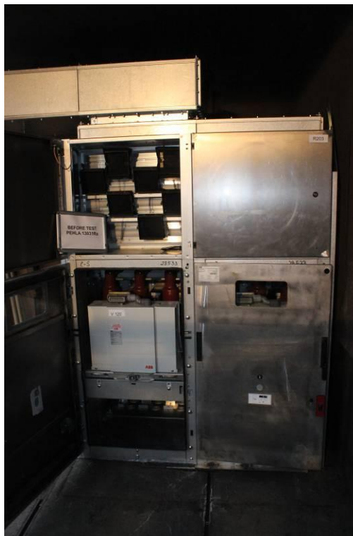
Photo No. 02 Before test PEHLA 13031Ra / 06 Test object, front view with doors of left-hand side panel opened.
