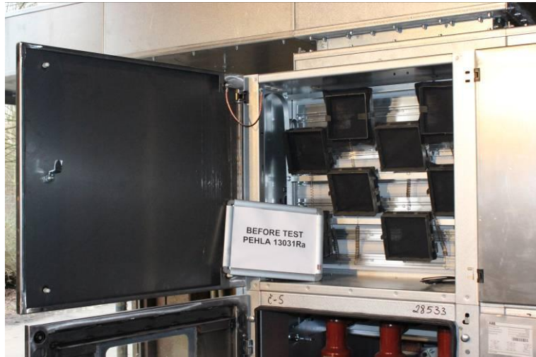
Photo No. 03 Before test PEHLA 13031Ra / 06 Additional indicators within low-voltage compartment
