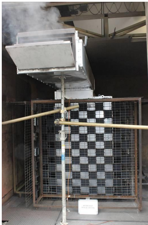
Photo No. 10 After test PEHLA 13031Ra / 06 Test object, side view with indicators and opened hatch at the end of the outlet
