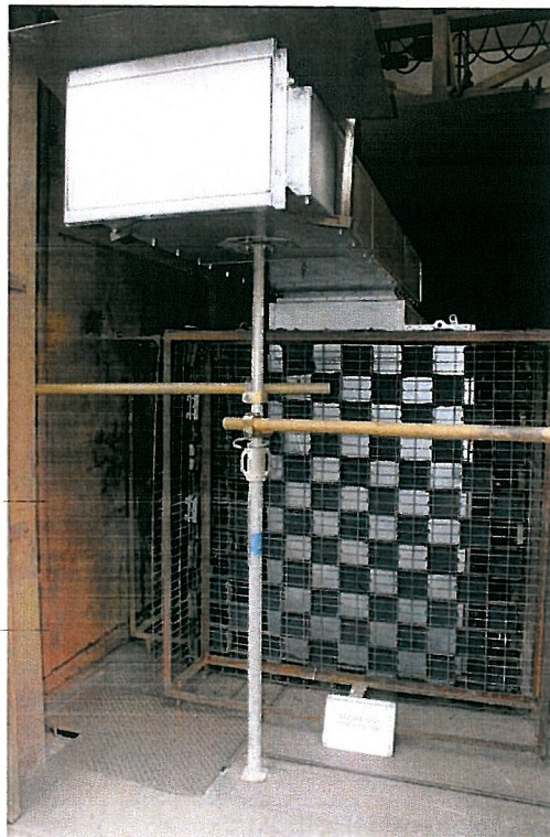
Photo No. 08 Before test PEHLA 13031Ra / 06 Test object, side view with indicators and closed hatch at the end of the outlet
