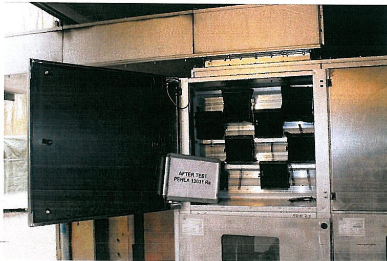
Photo No. 12 After test PEHLA 13031Ra / 06 Additional indicators within low-voltage compartment
