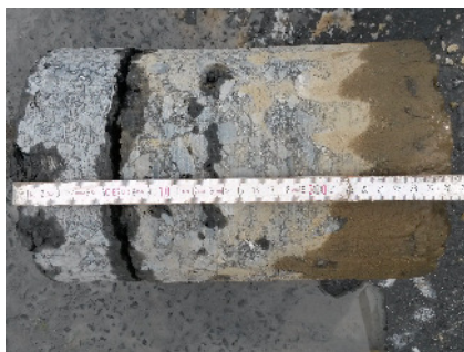
Foto 1: Asphalt Bohrkern (Dicke 28 cm)
