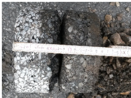
Foto 1: Asphalt Bohrkern (Dicke 16 cm)
