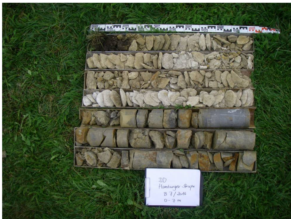
Foto 7: Bohrung B 7/2016, Bohrkern 0 – 7 m
