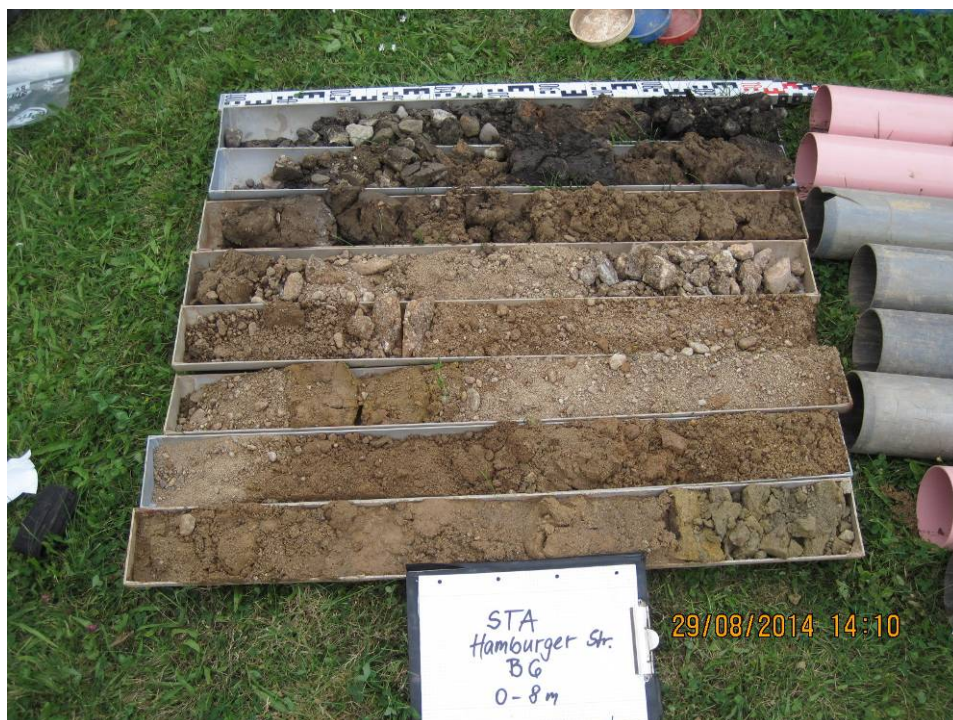
Foto 6: Bohrung B 6/2014, Bohrkern 0 – 8 m
