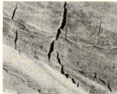
Figure 13. Stress corrosion cracks in weld in low strength electrode weld bend specimen exposed in ammonia with 10 ppm oxygen and 35 ppm water at -33°C (100x).
