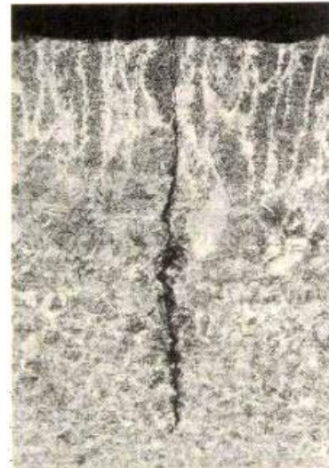
Figure 17. Stress corrosion crack in specimen from the cracked low temperature ammonia storage tank in Ludwigshafen (100x).
