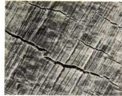
Figure 5. Stress corrosion cracks in tubular specimen exposed in ammonia with 1 ppm oxygen and 100 ppm water at -33°C (400x).
