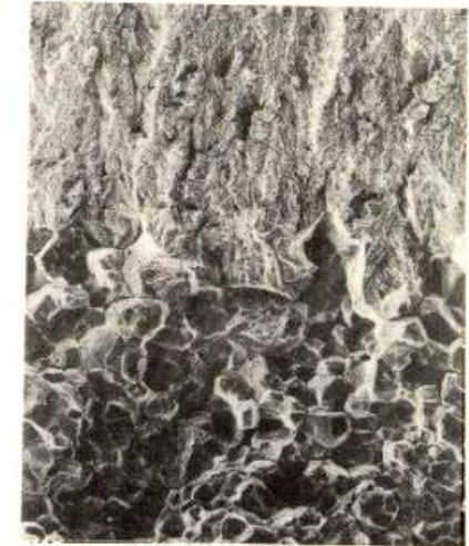
Figure 9. Transgranular cracking in weld metal (top) changing to intergranular in the heat-affected zone (bottom) (125x).
