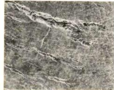
Figure 6. Stress corrosion cracks in tubular specimen exposed in ammonia with 10 ppm oxygen and 50 ppm water at -33°C. Cracks in the liquid phase, all cracks stop at the liquid/vapor interface (100x).
