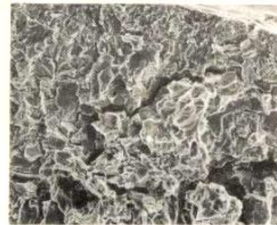
Figure 7. Transgranular SCC at 18°C (top right) followed by intergranular SCC at -33°C in compact tension specimen (500x).
