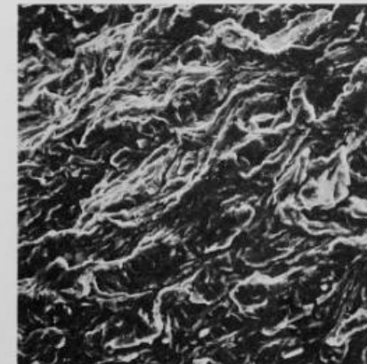
F) 9% Ni-STEEL FAILED BY SCC IN AMMONIA
