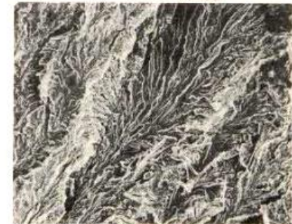
Figure 18. Fracture surface of stress corrosion crack in specimen from the cracked low temperature ammonia storage tank in Ludwigshafen (500x).
