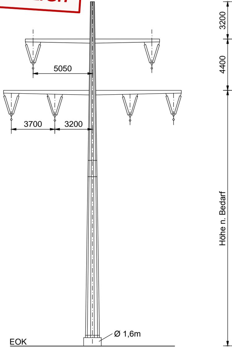
Stahlvollwandmast T1 + T2
