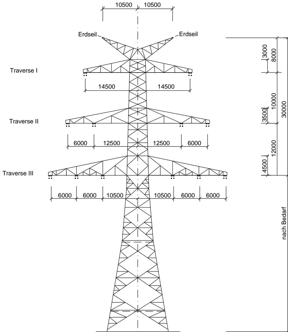
Winkelabspannmast WA160; DD-4-DE-2008.1
