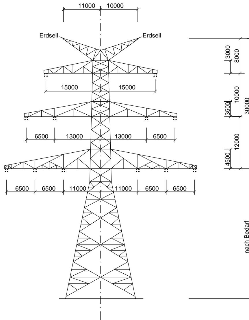
Winkelabspannmast WE/WAdiff140; DD-4-DE-2008.1
