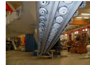
Jetting Nozzle and protective ring
