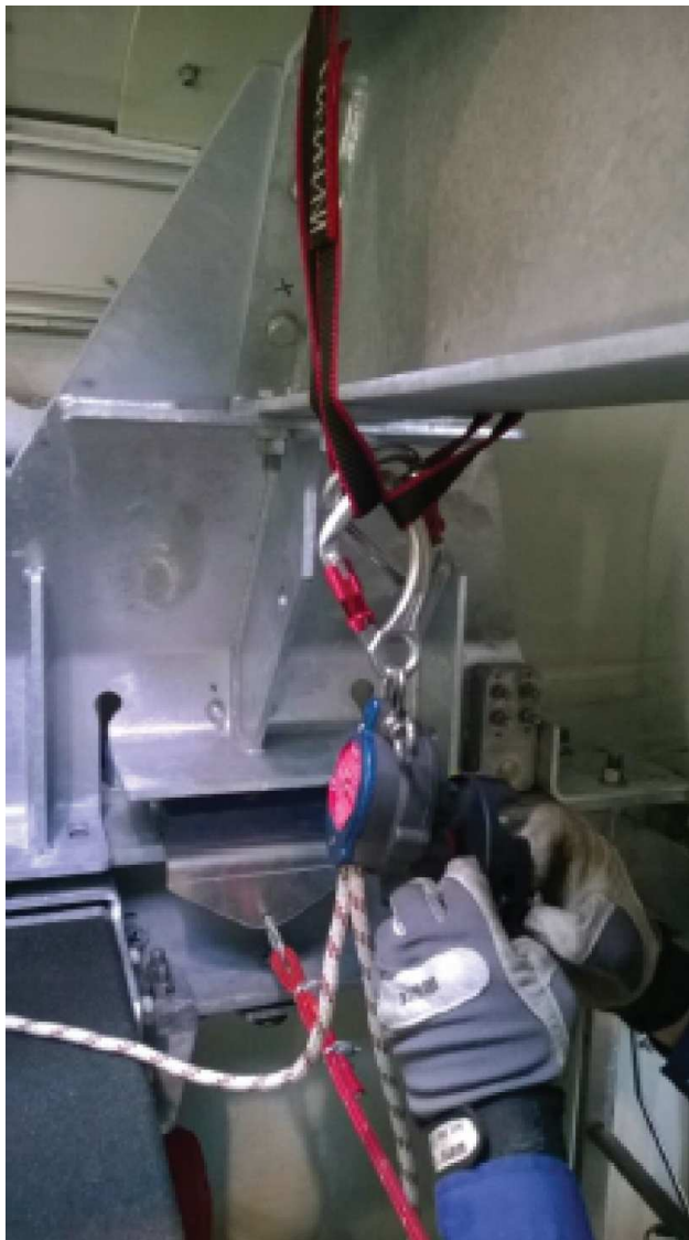
Figure 7.20: Descent unit device attach the to the moveable beam
