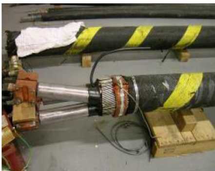
Figure 3. Assembling of the HV tricore cable inside the laboratory.
