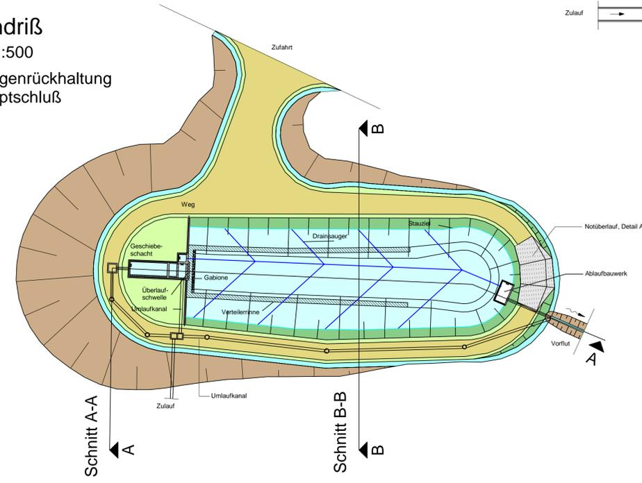
\* RBFA = Retentionsbodenfilteranlage
