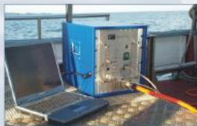
Parametric Sub-bottom Profiler SES-2000 compact during operation
